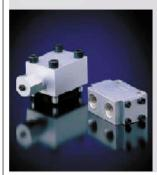
These valves are used for applications where one pump is required to supply two unevenly loaded consumers which must be driven simultaneously and independently (type TQ) or if one actuator requires priority flow (type TV).
