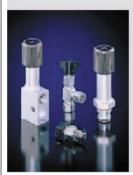
pressure by means of a slot with a constant width where the area of opening varies proportionally with the distance of the adjustment travel. Valves using this throttling principle are much less sensitive to contamination.
